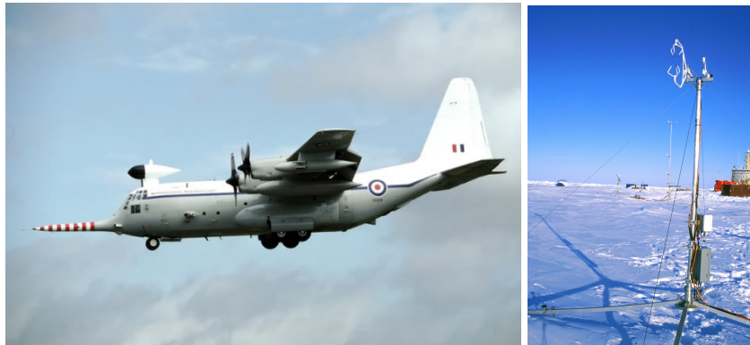
Figure 4.1: The UKMO Hercules C130 research aircraft. The photo on the right is taken during the Surface Heat Budget of the Arctic Ocean (SHEBA) experiment and show a sonic anemometer installed on a 2 m mast on the Arctic sea ice. In the background the icebreaker 'Des Groseilliers' is visible.
