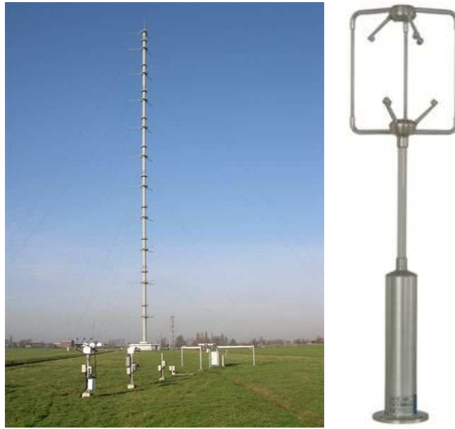
Figure 3.1: On the left a picture of the tall measurement tower of the KNMI at Cabauw is shown. This site is located on a height of 0.7 m below sea level at the coordinates 51^{\circ} 58' N latitude and 4^{\circ} 54' E longitude. The sonic anemometers at 60 m, 100 m and 180 m are placed on beams pointing south east from the tower. The sonic anemometer at 3 m height is placed 200 m north of the main tower. All sonic anemometers are of the type Gill R3 (Bosveld, 2008 - 2009). On the right a Gill R3 sonic anemometer is shown.
